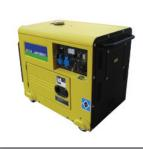
AC Rated Power ....: 4,2 kW AC Max. Power.....: 4,5 kW AC Voltage .....: 230 V AC Rated Current ...: 18 A Fuel Tank Capacity.: 16 lt. Oil Capacity.....: 1,65 lt. Fuel Consumption ..: 1,33 lt./hour Dimension (LxWxH).: 960 x 580 x 760mm Weight ...... 170 kg Starting Type .....: Electrical Start
